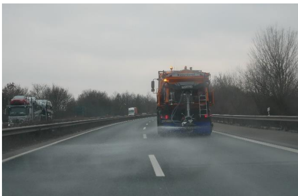
Figures 22 and 23: Application of 15 g/m 2 salt (fine grained) with a spreading width of 6 m at 50 km/h, left: prewetted salt FS30, right: dry salt.
