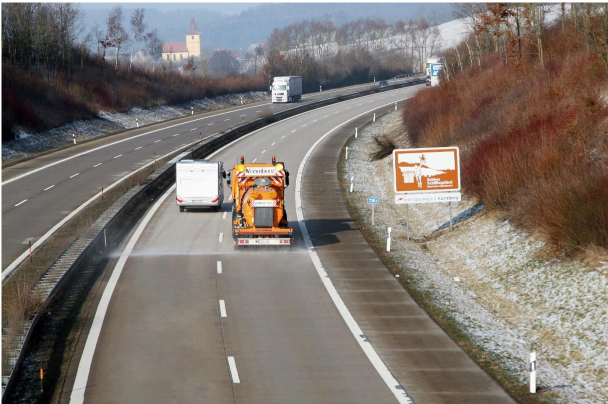
Figure 31: Direct brine application with a “Full wet” spreading machine
