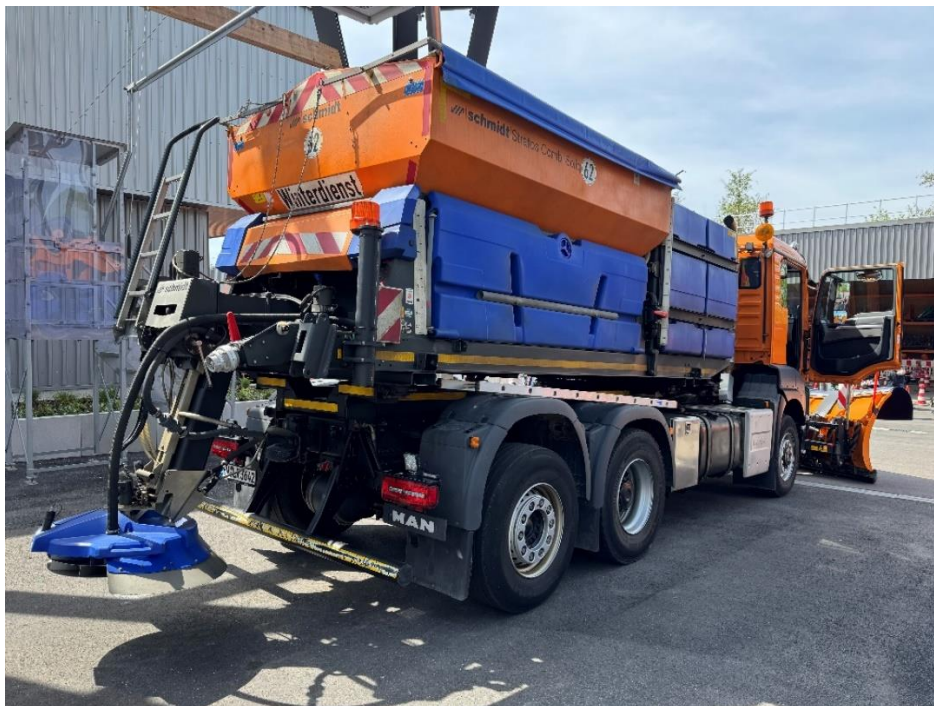
Figure 27: Combi spreader with spreading disc for direct brine applications on roadways up to 8 m wide
