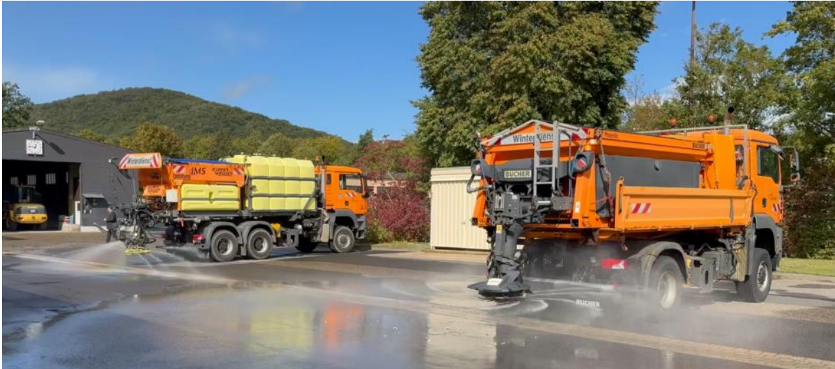
Figure 30: Direct brine application with combi spreaders (left: with spray nozzles, right: with rotating spray unit)
