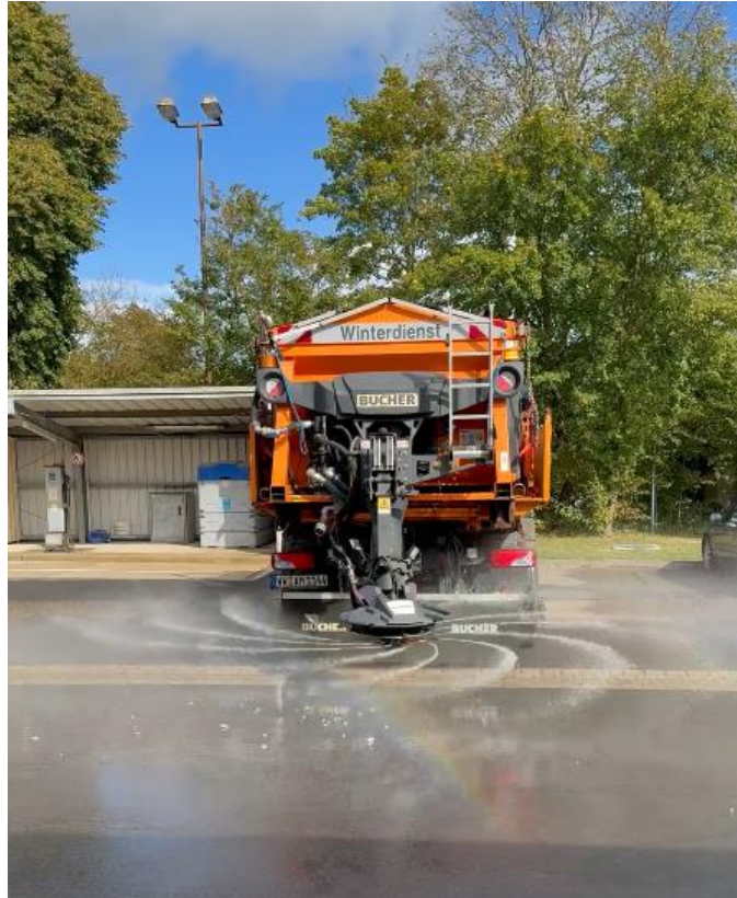
Figure 28: Combi spreader with rotating spray unit below the spreading disc for direct brine applications on roadways up to 12 m wide
