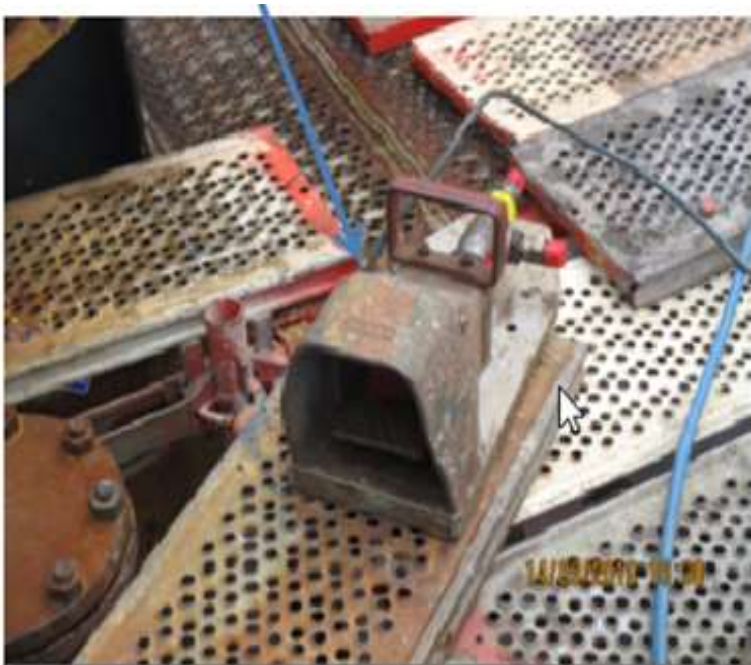
Figure: Demonstration of a technique that was potentially used to block foot pedal
