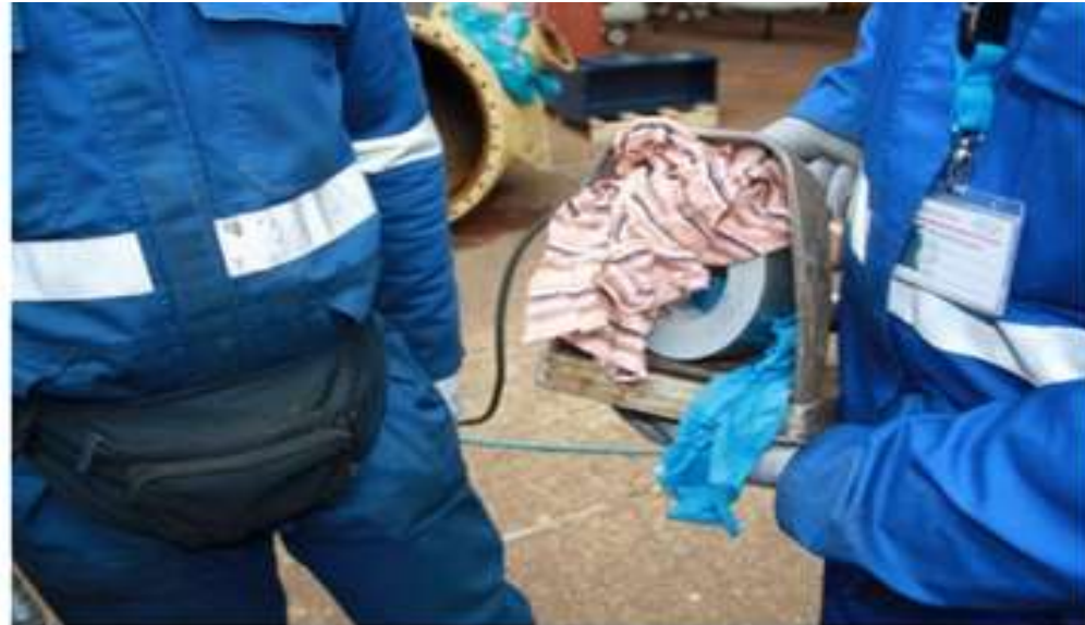
Figure: Demonstration of a technique that was potentially used to block foot pedal
